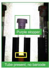
Automatically classify test tubes and cap type along with determining the liquid level.
