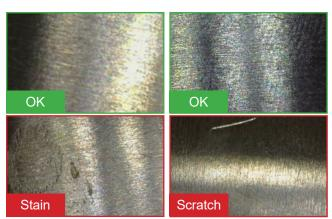
Leverage edge learning technology and machine vision to detect and classify imperfections, as well as differentiate between flaws and acceptable anomalies.
