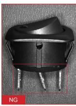
Check the quality of connector prongs on electronic components with edge learning tools.
