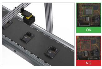
Vision systems embedded with edge learning verify correct assembly of PCBs.
