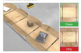
Vision systems with edge learning detect the hygiene of trays, as well as items stuck within cross-belt sorters or conveyors. These insights help prevent equipment damage or delays in processing.
