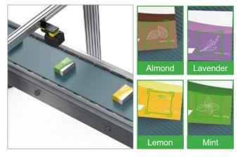
Classify and separate products based on size, color, and visual characteristics using edge learning tools.
