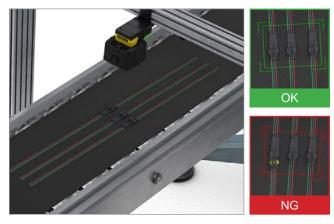
Vision systems embedded with edge learning can verify if connectors have been properly inserted in wiring harnesses.
