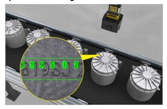
Vision systems with edge learning instantly read codes and direct part markings, even in low-contrast conditions and when the code is damaged.
