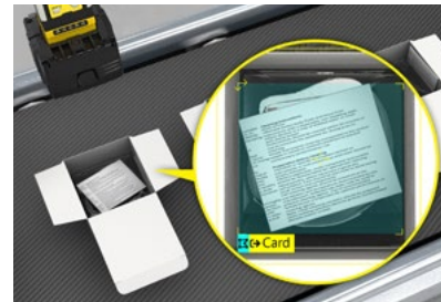
Verifying the presence of components such as clips, screws, springs, labels, seals, manuals, inserts, or accessories
