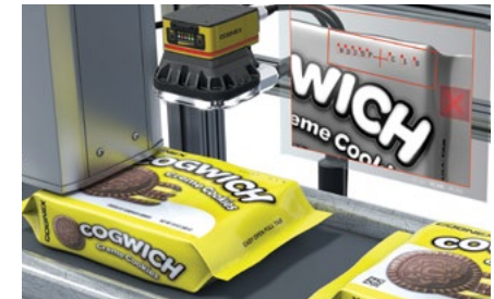
Checking if a sell-by date or lot number is printed correctly (OCV)
